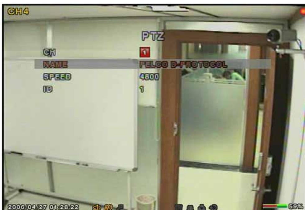
Figure 3.4.3. PTZ setup screen
