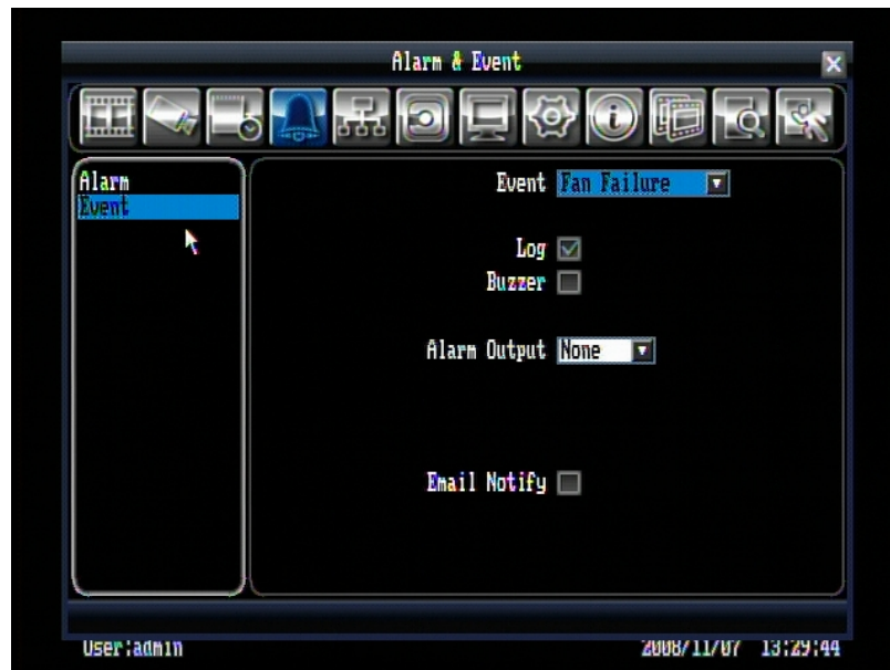
Figure 5.13 (Alarm & Event Menu – Event-Fan Failure)
