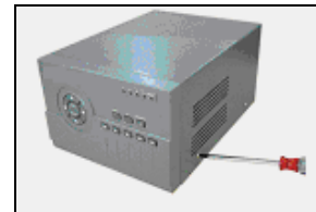
6. Close the top cover and screw it back on
