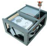
5. Assemble HD Bracket
