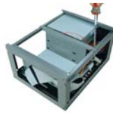
2. Dismantle the HD Bracket
