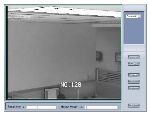
By default, the entire screen is set as motion detection area where is indicated with green border around the image. To mask a specific area, you
