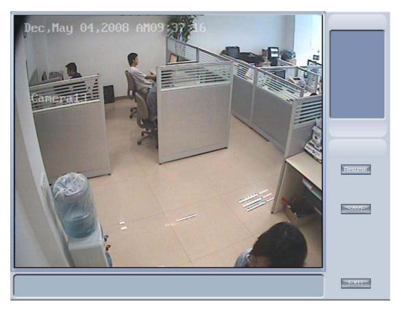
OSD include time and channel name. you can drag time or channel name to where you want directly in screen ,then press button to save it or press button to resume time and channel name to default position.
