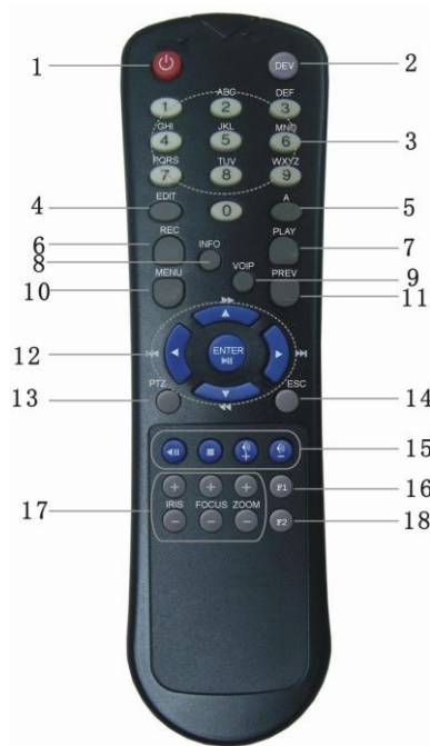
Fig. 3.2 Elevation of IR remote control
